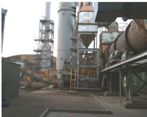
A process of directly heated thermal desorption (DTD) is being used to treat the soil in the contaminated areas.
